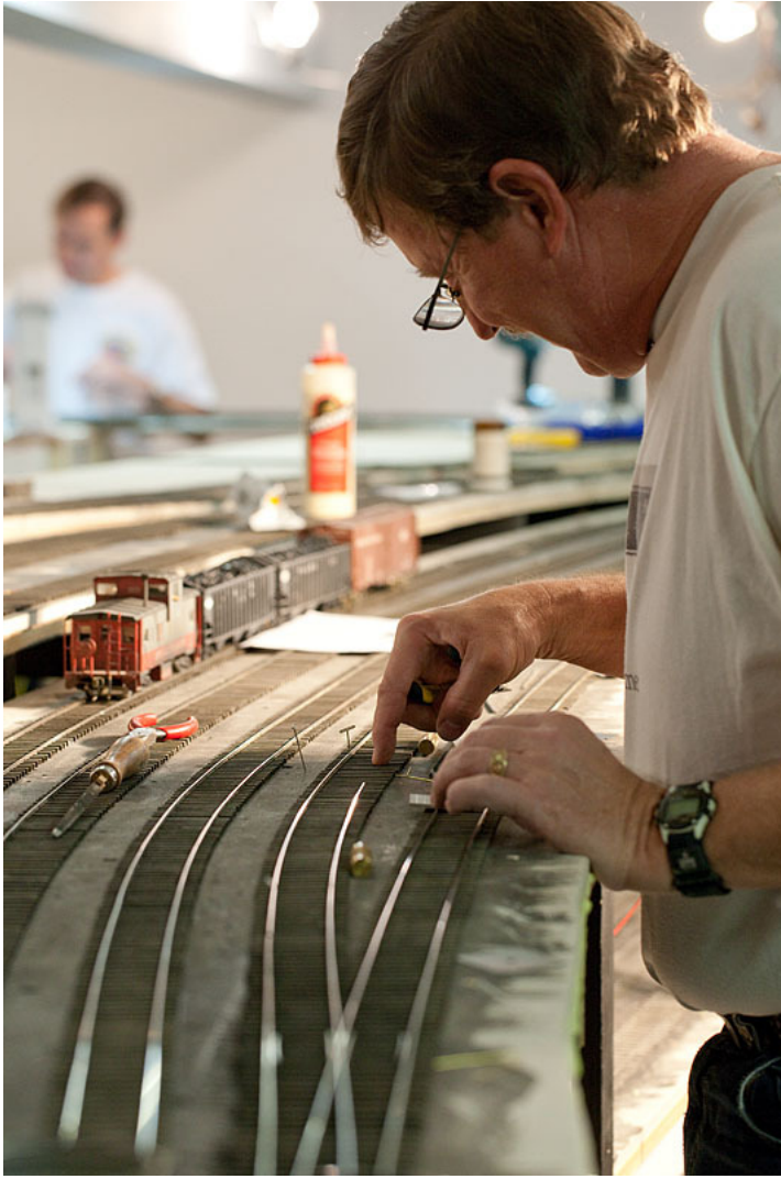
Mark spikes rail using the Tres Amigos rolling track gage
