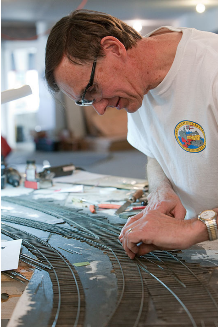
Trackwork in Havens yard, A/D tracks. For the record these are approximately #10 frog angle.
