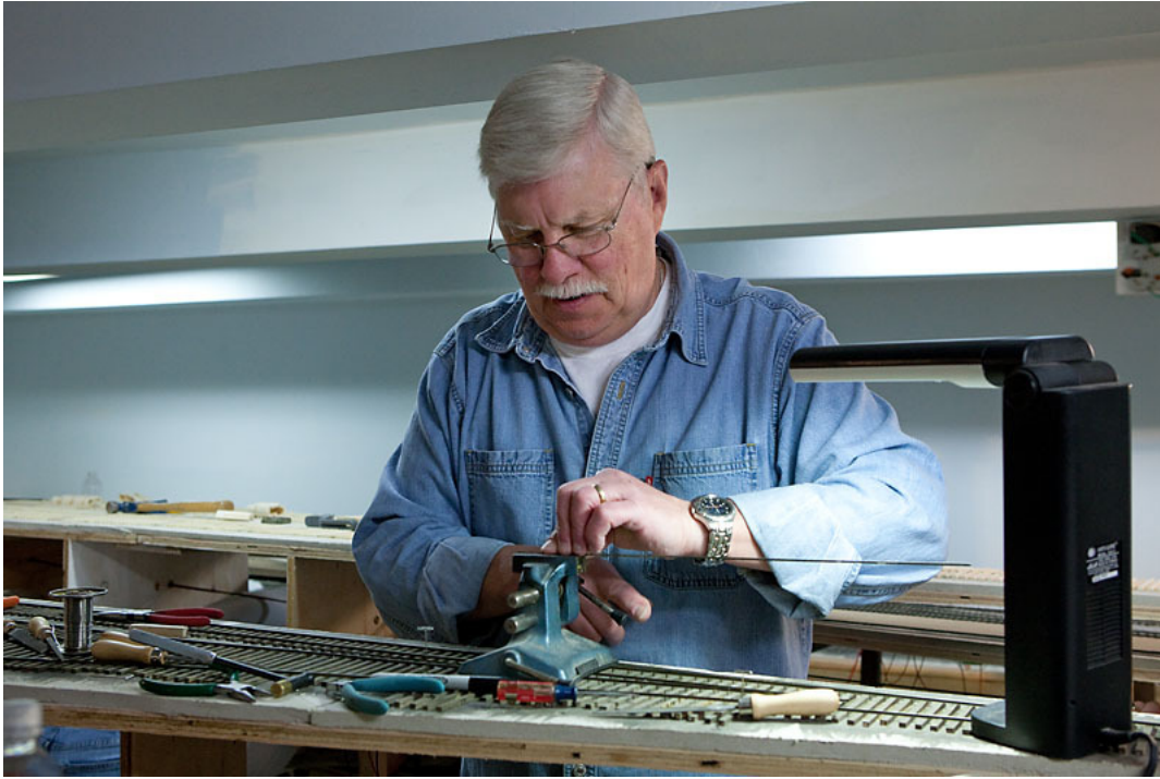
Levi connecting Havens yard rail feeder wires to the DCC power bus.
