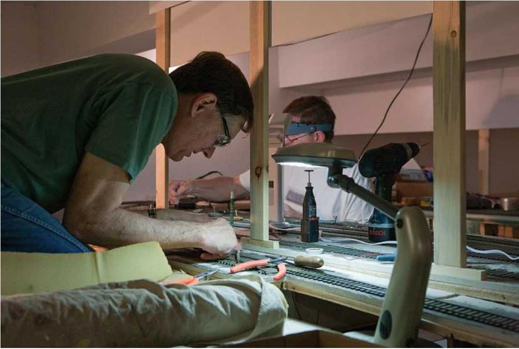
Jackson grinding a code 100 stock rail for a turnout in Fillmore Heights.
