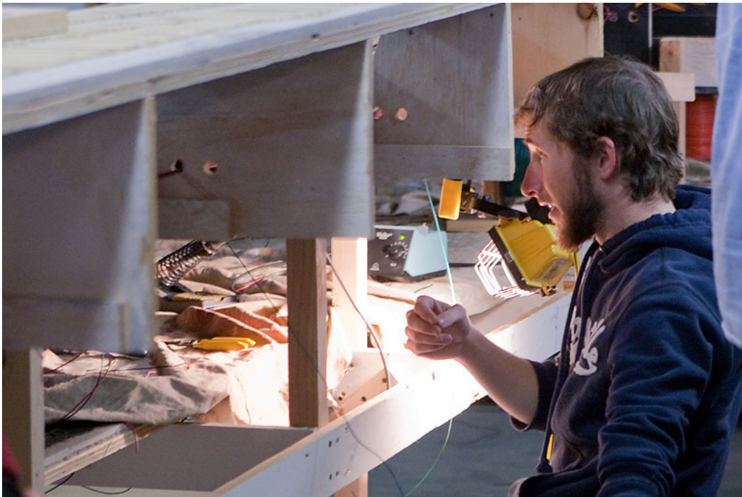
Craig wiring turnout motors.
