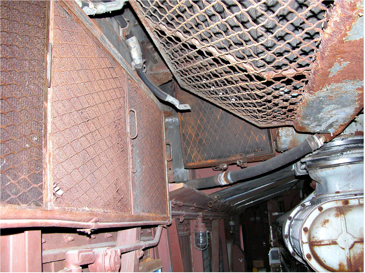
Dynamic brake squirrel cage fan on one side of the ARHS F3. There are two of them:
